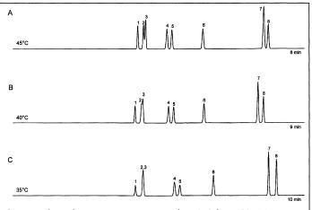
**Figure 1.** Solvent chromatograms at 45, 40, and 35°C. Column, DB-WAX 30 m × 0.32-mm i.d. (0.5-µm film thickness); split injector, 250°C, 100:1 split ratio; FID detector, 300°C; helium carrier gas, 32 cm/s; column temperatures, (A) 45°C for 5 min, 45–115°C at 10°/min; (B) 40°C for 5 min, 40–110°C at 10°/min; (C) 35°C for 5 min, 35–105°C at 10°/min. Peaks: 1, ethyl acetate; 2, isopropyl acetate; 3, methyl ethyl ketone; 4, isopropanol; 5, ethanol; 6, propyl acetate; 7, toluene; 8, 1-propanol.
